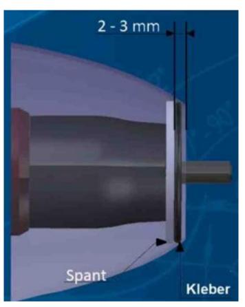
In the case of particularly large engines, a support motor frame must be installed for additional mounting
