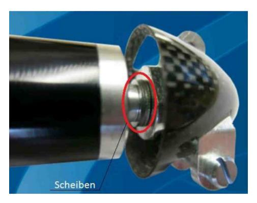
Please select the number of washers so that the spinner does not drag on the fuselage. There should be at least 0.5-1mm distance between spinner and fuselage.
